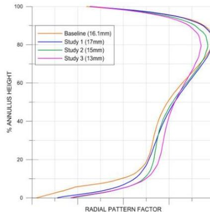
Figure 7. Radial temperature profile [6]
