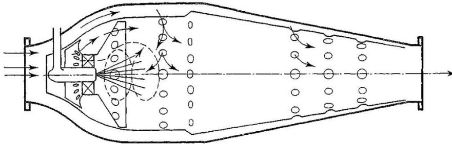
Figure 4. Recirculation zone in combustor equipped with swirler [2]
