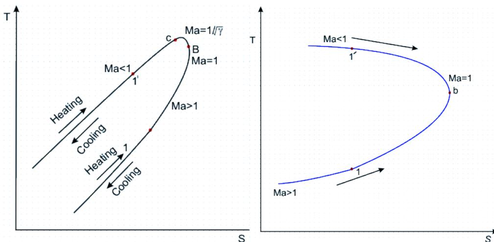
Figure 8. Rayleigh line (left) and Fanno line (right) [6]
