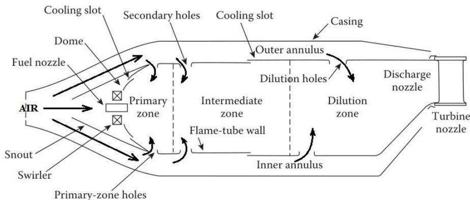
Figure 1. Main components and combustion zones of a conventional combustor [1]
