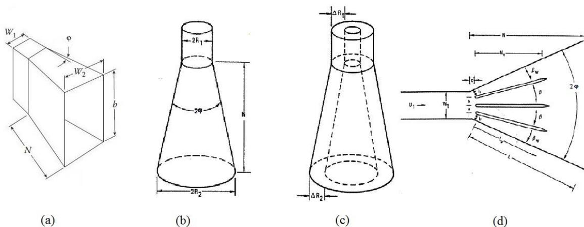
Figure 3. (a) Two-dimensional diffuser; (b) Conical diffuser; (c) Annular diffuser; (d) Vaned diffuser [4]
