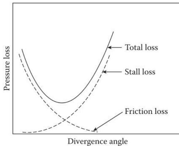
Figure 2. Influence of divergence angle on pressure loss. [1]
